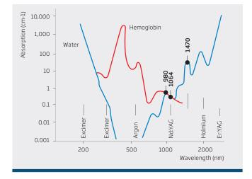
Through the occupation of the absorption maxima and minima by the diode laser of wavelengths 980 nm, 1064 nm and 1470 nm, we succeeded in adapting the penetration depth to the extent of the thyroid nodule to be treated.
